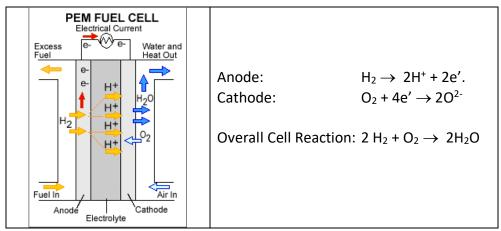
The PEM is the Proton Exchange Membrane. It allows H+ ions to move through the membrane, forcing the electrons along the conductor. There are also hydrogen fuel cells that are alkaline (OH- is the electrolyte) and cells that are acidic (phosphoric acid is the electrolyte).
